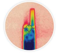
Infrared analysis shows major conductivity in aluminum and virtually none with Innergy\*
